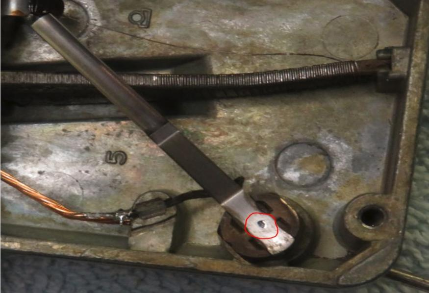
I used a 5/32" punch and a hammer to push the dimple farther into the inside of the cover plate. I moved the dimple .003". (Note: I positioned both dimples over small holes in a piece of wood when using the punch to avoid bending the cover plate and avoid flattening the dimple being punched.)
