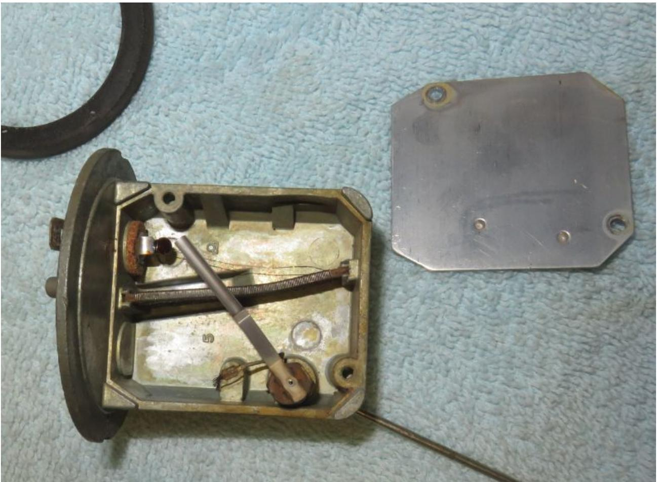
The sender has a braided cable to connect the wiper arm to the housing body. From what I could tell with my multimeter, the braided cable was not making a good connection anymore. The braided cable was just pushed into the slot via some high force press. No weld or solder used.
